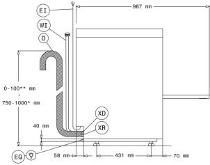
ΕI Electrical inlet (power) EO **Electrical Outlet** HWI Hot water inlet Rinse aid connection
